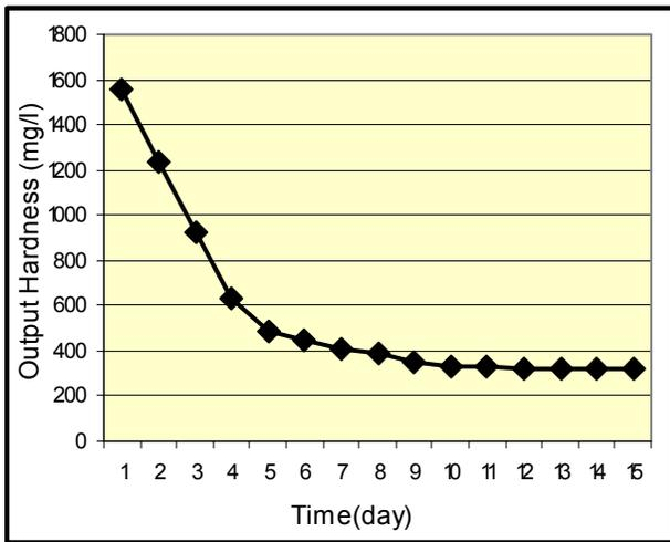
Fig. 6: Hardness variations in effluent water (in constant input hardness: 300 mg/l)
