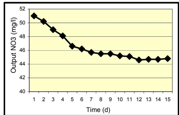
Fig. 4: Nitrate variations in effluent water (in input nitrate:  $45.5 \text{ mg/l}$ )
