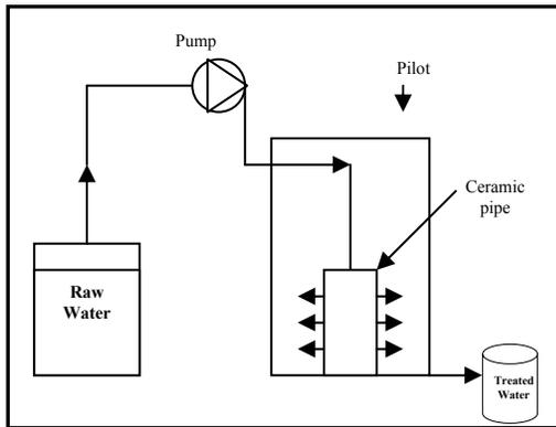
Fig. 1: Schematic design of the pilot
