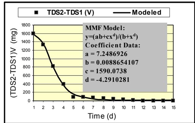
Fig. 3: Calculated amount of salt released in discharge water by mathematical model
