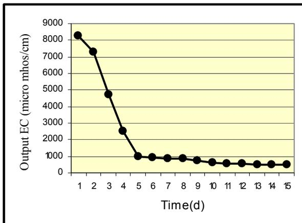
Fig. 2: EC variations in effluent water (in constant input EC:  $500 \mu\text{mhos/cm}$ )
