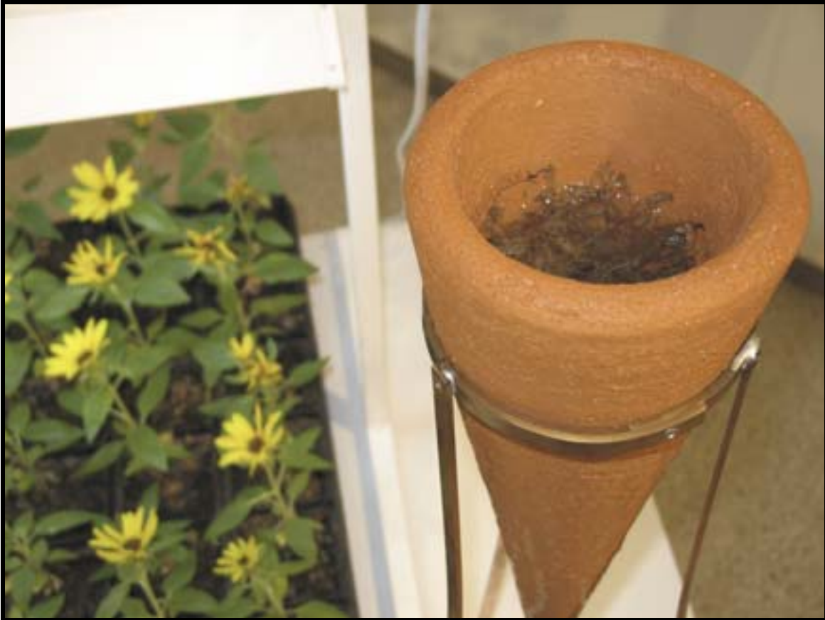
Grow , detail; dirty water inside of terracotta-coffee-clay water filter
